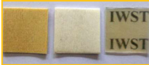
Natural wood (Left most), Lignin modified wood (middle) and Transparent wood (right most) placed on a paper with letters "IWST"
