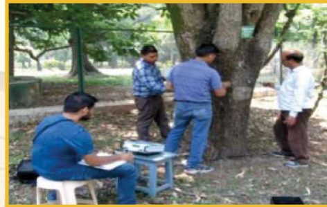
Measurement of hollowness in a tree using ultrasonic detector
